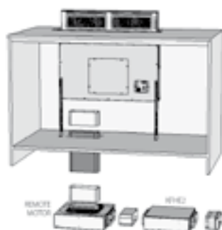
S-KFHE2 HIGH EFFICIENCY FILTERING KIT FOR KITCHEN PLINT MIN. 100mm HEIGHT
